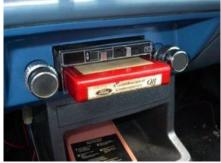
track to cassette tapes. Speakers went from one in front and maybe one out back, to a pair of 6x9s in the back and a set in either the door panels or a small pair in the kick panels or dash. Real audio fans added equalizers,
