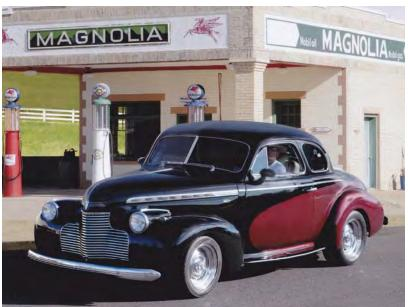
"Rachel" has been converted from hot rod to street rod -mods, i.e. Chevy 350/330 hp crate motor, 700-R4 overdrive, '68 Chevy 308 rear end, rack/pinion with aftermarket coil-over shocks, Vintage Air A/C.
